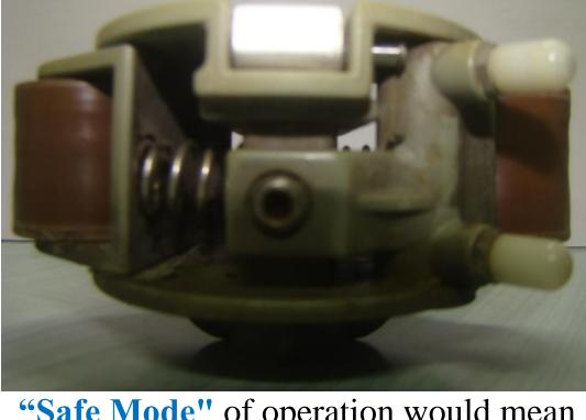
**"Safe Mode"** of operation would mean disabling the Arterial blood pump, clamping the venous line, and stopping UF, thus isolating the patient by all blood alarms (air detector, arterial, venous, blood leak, transmembrane pressure, blood pump torque). Venous pressure Measurement port Ultrasonic Air Detector Line Clamp Optical Detector
